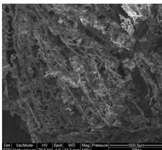
**Figure 1:** SEM image of biomineralized gelatin-based scaffold with an aligned channel-like porosity.
