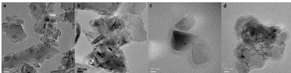
**Figure 1.** TEM micrograph of pristine (a) cNDs, (b) MPEG-PCL-modified cNDs, (c) pristine rFNDs and (d) MPEG-PCL-modified rFNDs. Scale bar: (a,b) = 20 nm; (c,d) = 10 nm.
