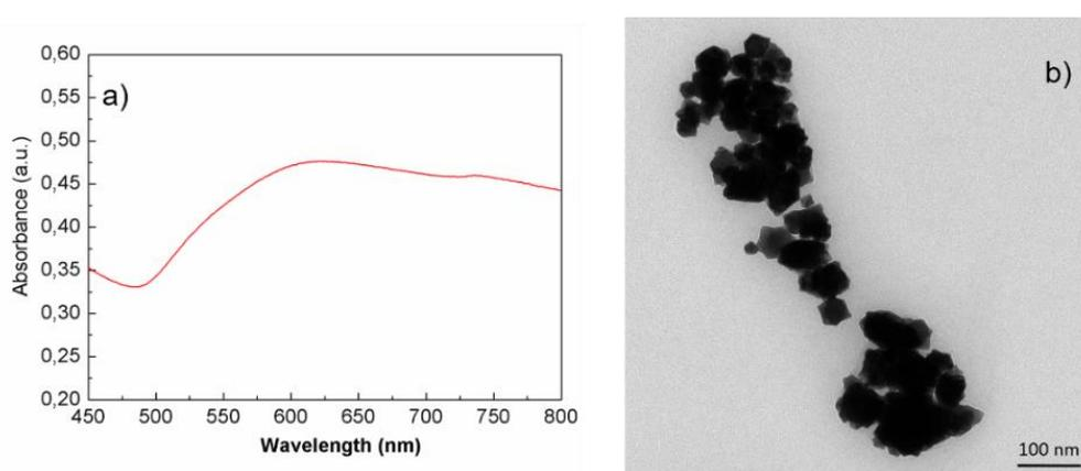
**Figure 1.** Au nanocrystals VIS spectrum (a), and TEM micrograph (b)
