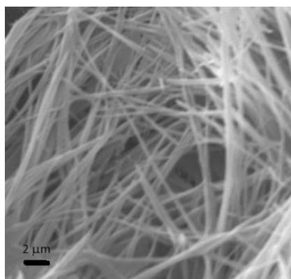
**Figure 1.** SEM micrograph of FmocFGFF hydrogel.
