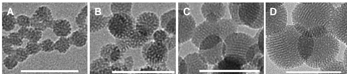
**Figure 1.** TEM images (scale bar 100 nm) of MSNs (average diameters: A – 25 nm; B – 38 nm; C – 55 nm; D – 70 nm).
