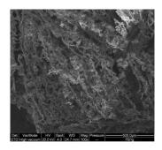
**Figure 1**: SEM image of biomineralized gelatin-based scaffold with an aligned channel-like porosity.
