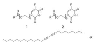
Chart 1. Molecular structure of non-ionic diacetylenic surfactant 1 and 2.
