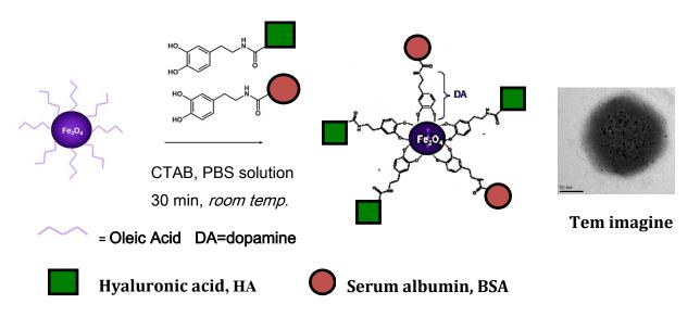
**Figure 1.** BSA-HA@Fe<sub>3</sub>O<sub>4</sub> preparation
