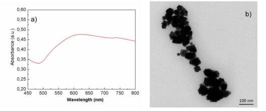
Figure 1. Au nanocrystals VIS spectrum (a), and TEM micrograph (b)
