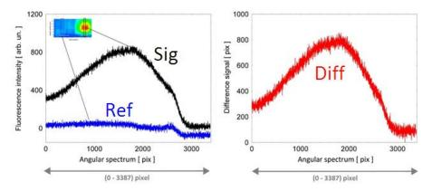
**Figure 1.** Fluorescence spectra obtained at the end of the bio-recognition assay in the reference (absence of the cancer biomarker, blue curve) and signal (presence of cancer biomarker, black curve) regions, respectively. The red spectrum is the differential signal.
