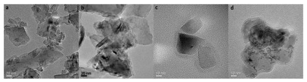
**Figure 1.** TEM micrograph of pristine (a) cNDs, (b) MPEG-PCL-modified cNDs, (c) pristine rFNDs and (d) MPEG-PCL-modified rFNDs. Scale bar: (a,b) = 20 nm; (c,d) = 10 nm.
