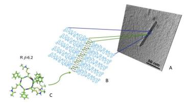
**Figure 1.** A) TEM micrographs of PEP8-Phe-PEG NPs; B) Structural model proposed for the corresponding NPs; C)  $\beta$ -like conformation with a 6.2 residues per turn preferred by the linear DL-octapeptides.
