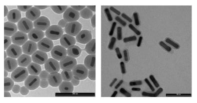
**Figure 1.** TEM images of GNRs coated with a 30 nm of  $SiO_2$  shell (left) and GNRs coated with a 10 nm of mixed oxide  $SiO_2$ -TiO<sub>2</sub> (right).
