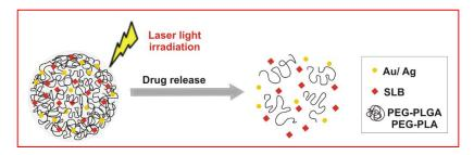
**Figure 1.** Schematic representation of the stimulated laser light drug release from the metal/polymer nanocomposites.
