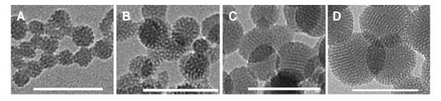
Figure 1. TEM images (scale bar 100 nm) of MSNs (average diameters: A - 25 nm; B - 38 nm; C - 55 nm; D - 70 nm).
