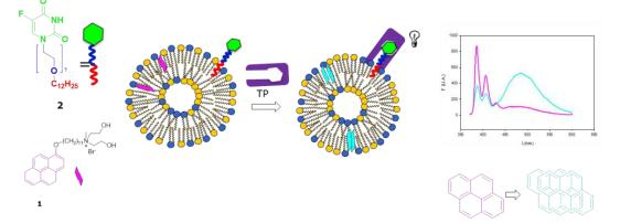
**Figure 1.** Liposome-based biosensor: the induction of an optical signal upon the interaction of liposomes functionalized with 5–FU derivatives with the target enzymes.
