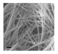
Figure 1. SEM micrograph of FmocFGFF hydrogel.
